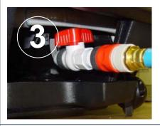
Screw the orange disconnect adapter to the male hose. Slide the orange quick connect onto the discharge valve. Make sure that the connection is secure.
